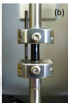
Figure 3: a. the DSR; b. the test setup; c. master curves of mortars at a reference temperature of 20°C
