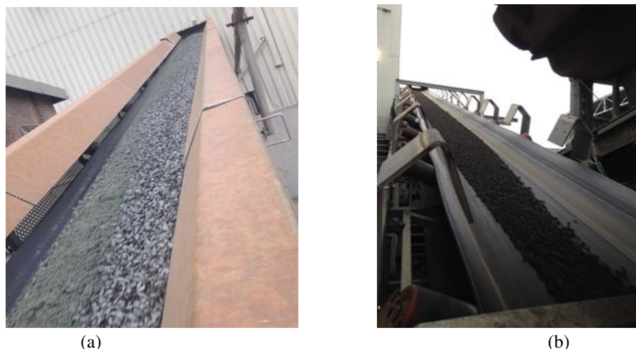
Figure 6: Production of porous asphalt with 25% PA-stone through white drum (a) or black drum (b)
